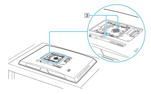
5 Flip over the mounting base plate (4) and screw it onto the back of the computer using the six screws (5) attached at the same place in step 3.
